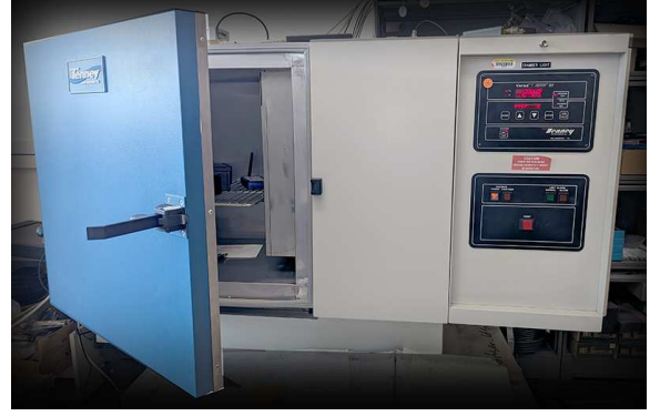
Fig. 4. The programmable thermal chamber
